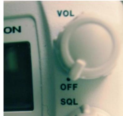
Why: Leaving the radio on will shorten the life of the display. If you forget to plug in the power cord, the radio will run down the battery. If you had the squelch on and the volume turned up loud, live-aboards nearby may be awakened in the middle of the night by radio traffic.
