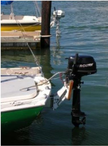
Do: Tilt the motor to the first position (**not all the way up**) on your boat **and** any of the surrounding boats whose motors you may have tipped down before you went sailing. The bottom end should clear the water by an inch or two.
