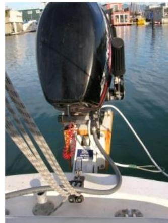
Why: The hose may deform permanently, causing a flow restriction. The hose can also be weakened, leading to a break in the fuel line (probably when someone needs it most).
