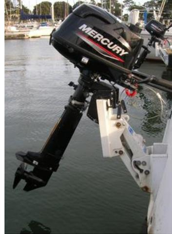
Why: Some of the motors will sit partly in the water when tilted down, even if the mount is raised. Immersion allows marine life to form and, more importantly, promotes corrosion.
