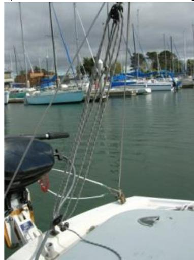
Why: Constant backstay tension puts strain on the mast and rigging, and they can develop a permanent set.
